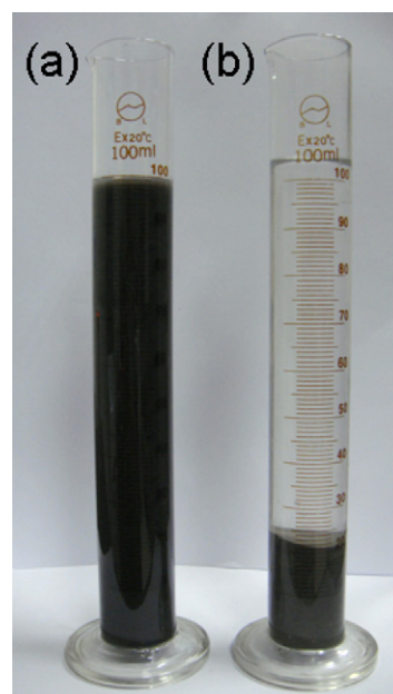
Fig. 13. Coal washing wastewater. (a) Before and (b) after treatment. (Conditions: 100 ml wastewater, adjusted the initial pH to 9 by CaO, FA-HCl-Y3 coagulant dosage 10\ g\ l^{-1} , 40 min treatment.)
